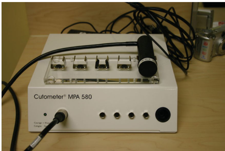
▲ FIGURE 38-3 The Cutometer. The black suction device is placed on skin to measure elasticity.
